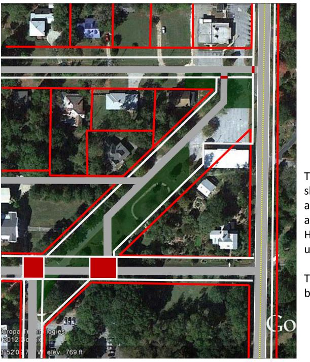
To improve safety, the city could shift the intersection of Whatcoat and Pierce Streets. This clears up ambiguity at the intersection with Haygood Street, and it removes unnecessary pavement.
