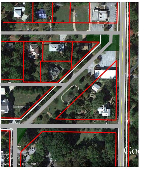
An easy first step is to remove unneeded pavement and to straighten George Street. This creates a "clean," green, and clearly delineated intersection.
